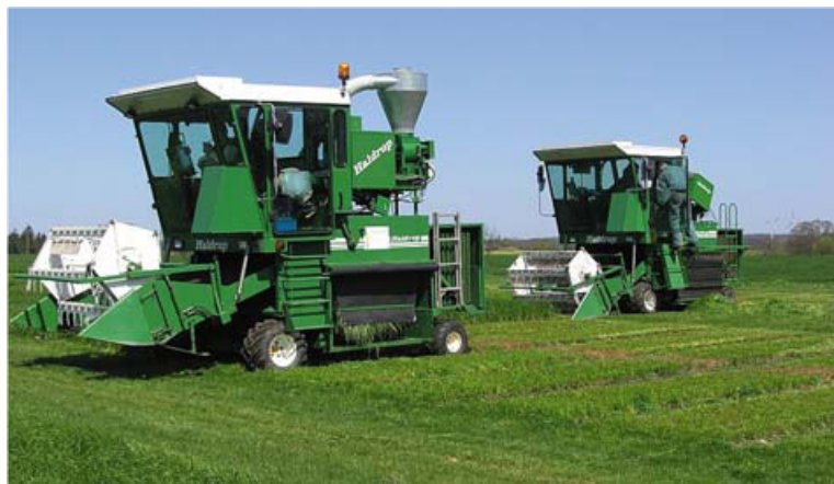
Figure 4. The plot harvester for forage is equipped with a sampling device and with a built-in Near-Infrared Reflectance Spectrometer for ,online‘ determination of the quality of forage (Photo U. Feuerstein)
