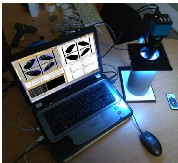
1 – video camera Video Microscope Camera 1080P 16MP manufactured by Eakins; 2 – sets of LEDs of three types (red, green, blue); 3 – personal computer; 4 – protective screen; 5 - seeds
